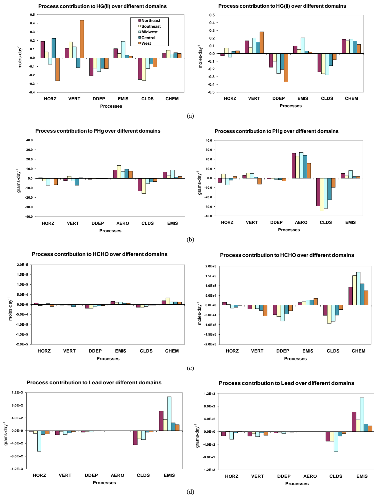
Figure 13. The monthly-mean contributions of individual processes to the concentrations of selected hazardous air pollutants: (a) Hg(II); (b) PHg; (c) HCHO; and (d) Particulate lead over different sub-regions of CONUS domain in January (left panel) and July (right panel) 2002. HORZ, VERT, DDEP, CLDS, CHEM, AERO, EMIS denote the processes of horizontal transport, vertical transport, dry deposition, cloud process, chemistry, aerosol chemistry, and emissions, respectively.
