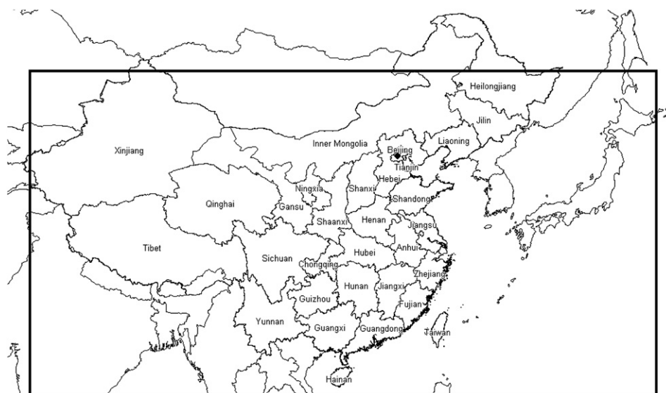
Fig. 1. The Models-3/CMAQ modeling domain at a horizontal grid resolution of 36-km (164 × 97 cells). The MM5 modeling domain is three grid cells broader on each side of the CMAQ domain. The diamond indicates the location of the continuous PM 2.5 monitoring site located in the campus of Tsinghua University (THU).
