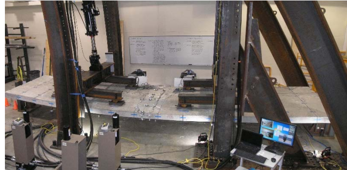
a) Beam test under deflection (Photo: SGH)
