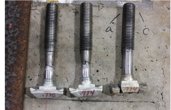
Fracture of the bolts
