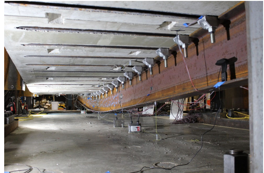
Composite beam test setup
