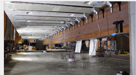
View Underneath Specimen Showing Clamps in Action
