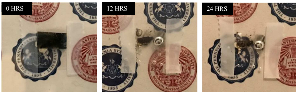
Figure S9 | Dissolution of the Zn electrode (taped to the petri dish) after being immersed in water for 0 hours, 12 hours, and 24 hours. Photo credit: H. Cheng, Penn State University® and Northeastern University®.
