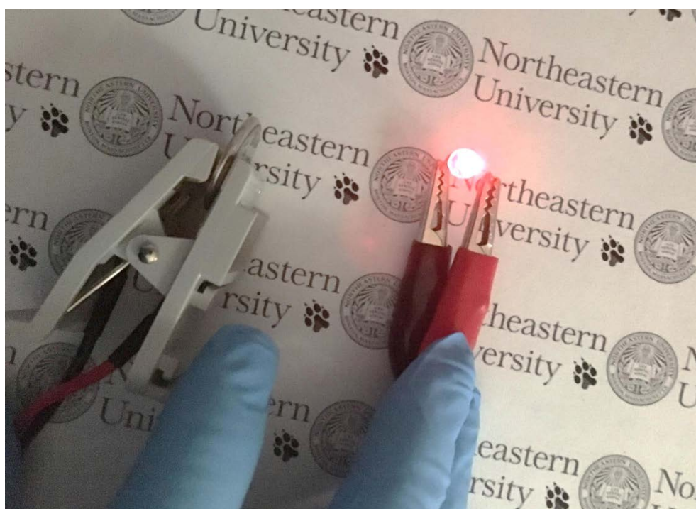
230 Figure S13. Optical image of a LED powered using the CNFF based PIB.
