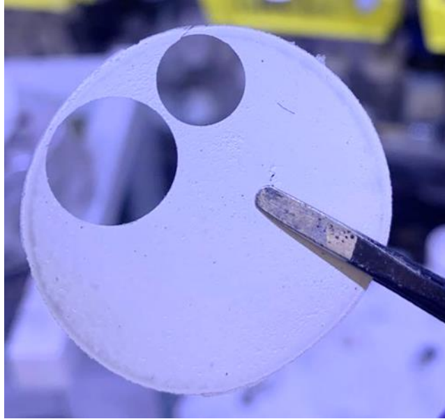
Fig. S5. Photo of SE membrane after punch to show the robustness.
