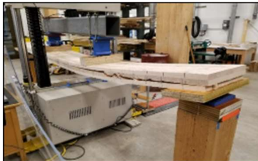
Figure 1B: Plank Testing of Novel CLT Lay-ups
