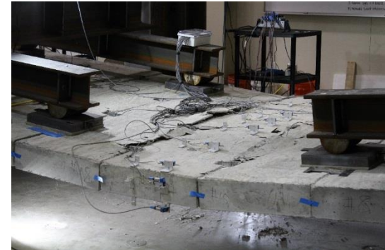
Localized concrete crushing
