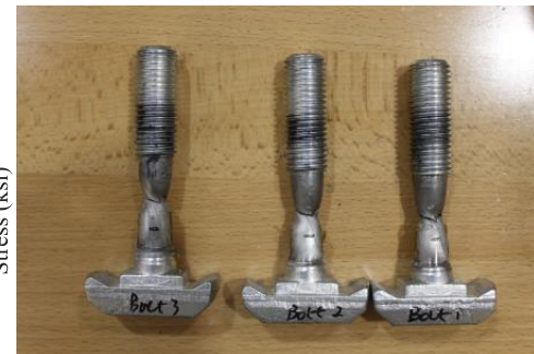
M20 bolts Fractured bolts
