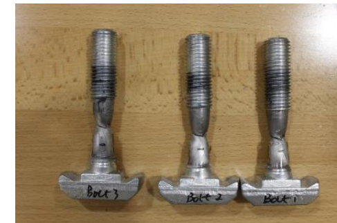
M20 bolts Fractured bolts
