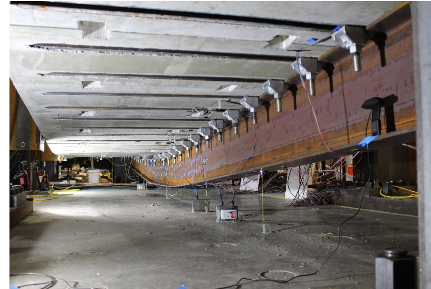
Composite beam test setup
