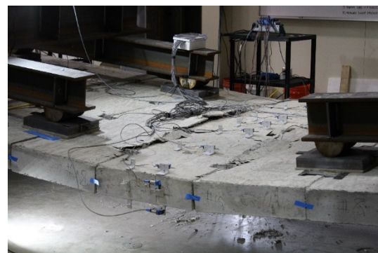
Localized concrete crushing
