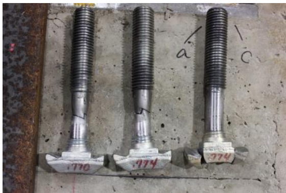
From right to left: Bolt1, Bolt2, and Bolt 3 a) M24
