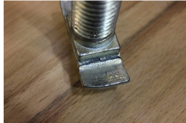
Bolt head fracture
