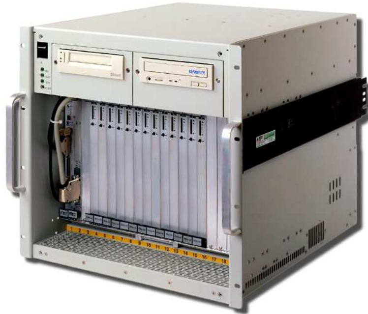
Figure 4.2: The 6U VME chassis supports Mercury’s Race++ backplane and accommodates ad-hoc configurations of PowerPC and FCN daughtercards.[42]
