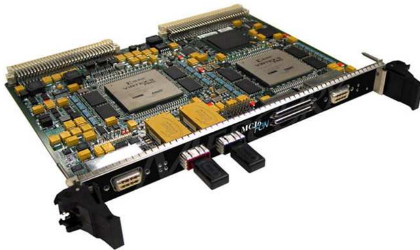
Figure 4.4: The FCN module houses two FPGA compute nodes based on the Xilinx Virtex II Pro 70 FPGA.[43]
