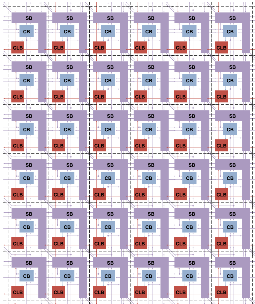
Figure 2.5 Representative block diagram of an island-style FPGA.
