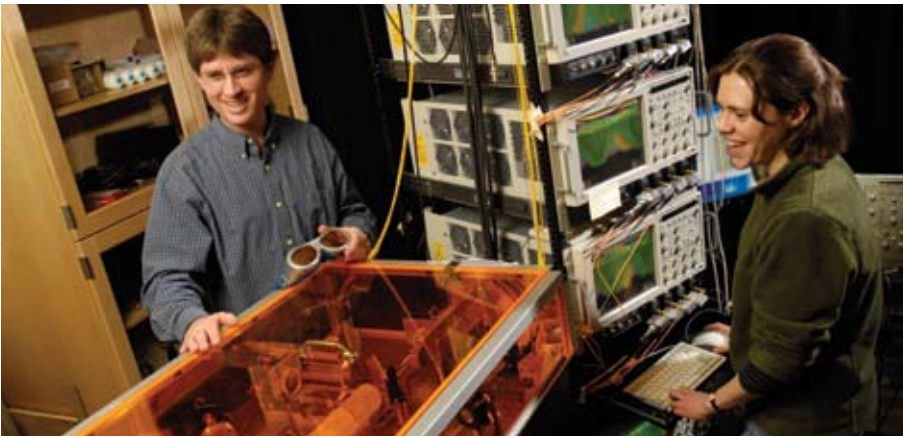
At Washington State University, an ALERT partner, Senior Project Engineer Kurt Zimmerman and an intern, Eryn Cook, work on the Institute for Shock Physics' Multipoint VISAR, which is used to make velocity measurements during experiments.
